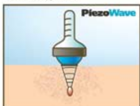
High-energy, focused shock wave * The maximum energy of the high-energy, focused shock wave is directly at the point of pain.
